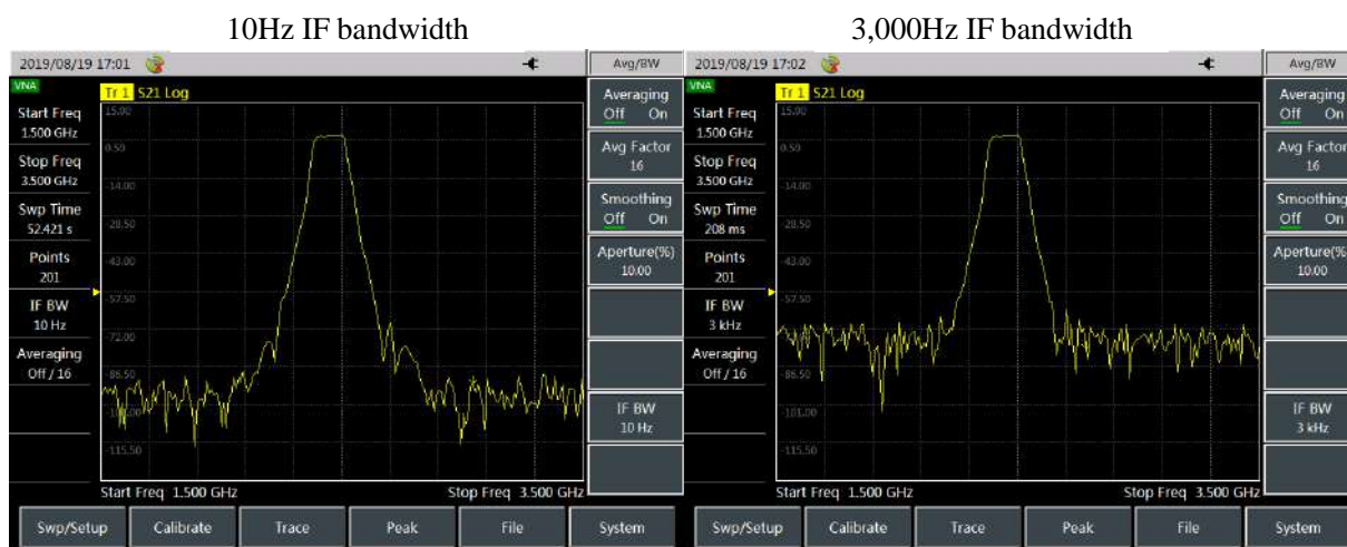
Figure 4-2 Effect of IF Bandwidth on Measurement Results
