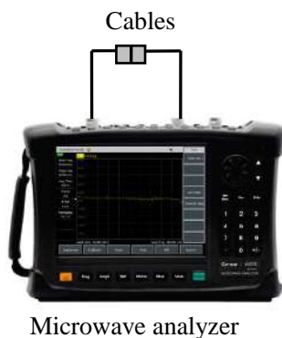
Fig. 4-4 Standard piece connection for transmission measurement response error correction
