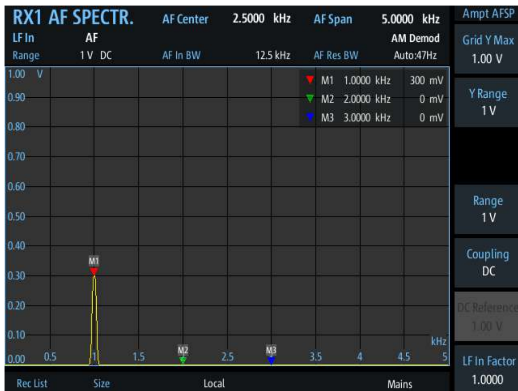
Figure 5-4: AF Spectrum for LF input
