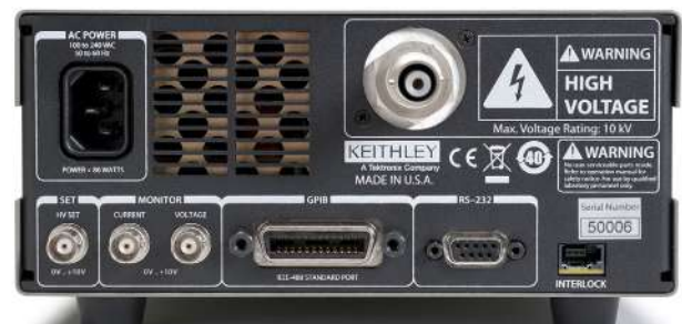
2290-10 rear panel showing the IEEE-488 interface connector, RS-232 interface connector, high voltage output connector, analog control/output connectors, and interlock connector.
