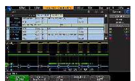
Figure 19. Multi-bus time aligned decode.
