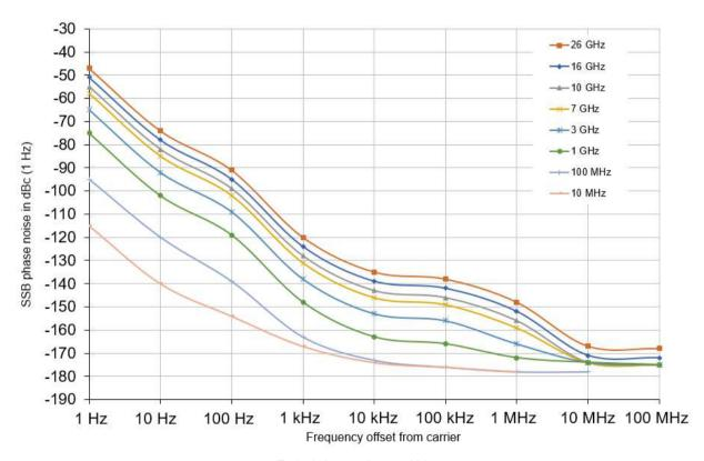
Typical phase noise sensitivity (start offset = 1 Hz, correlation factor = 1, signal level = 10 dBm)
