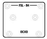
Generates a very precise 10 MHz reference signal. The signal is output at the EXT REF standard connector, see page "EXT TRIG/GATE" on page 27. The output level is listed in the data sheet.
