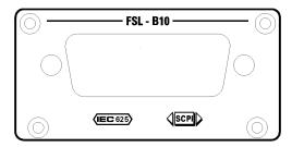
In compliance with IEEE488 and SCPI. Used to connect a computer for remote control, see also Chapter 6.1, "Preventing Electromagnetic Interference", on page 37.
