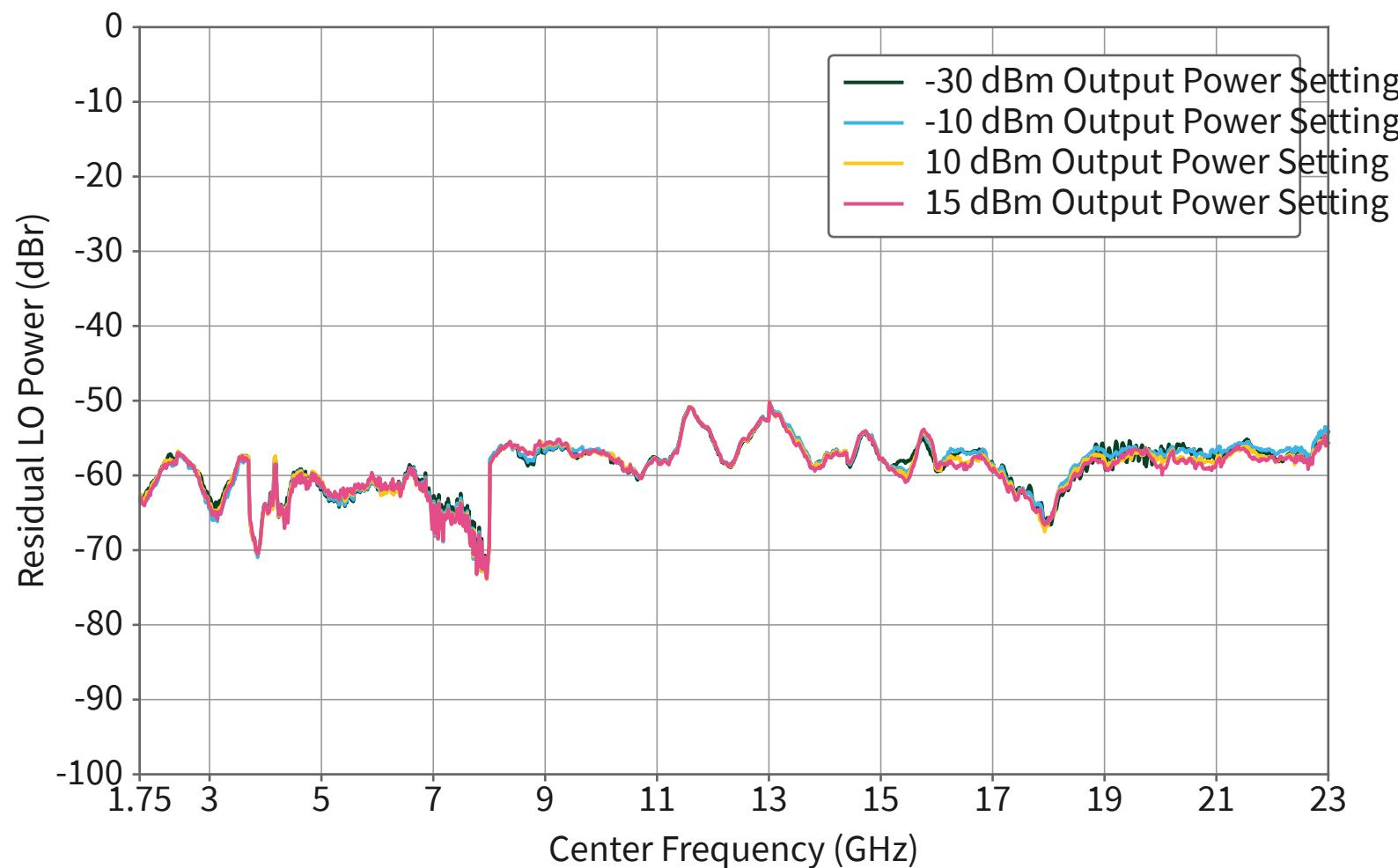
Conditions: Measured by sweeping a 0 dBr CW signal across the bandwidth and calculating the maximum residual LO power.
