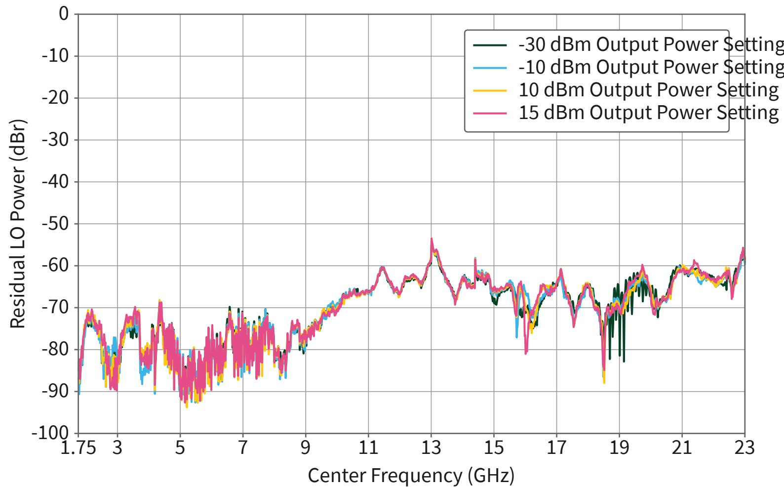
Conditions: Measured by sweeping a -12 dBr CW signal across the bandwidth and calculating the maximum residual LO bandwidth. A digital backoff of 12 dB is representative of the residual LO power performance for many wideband communications signals with a PAPR around 12 dB.
