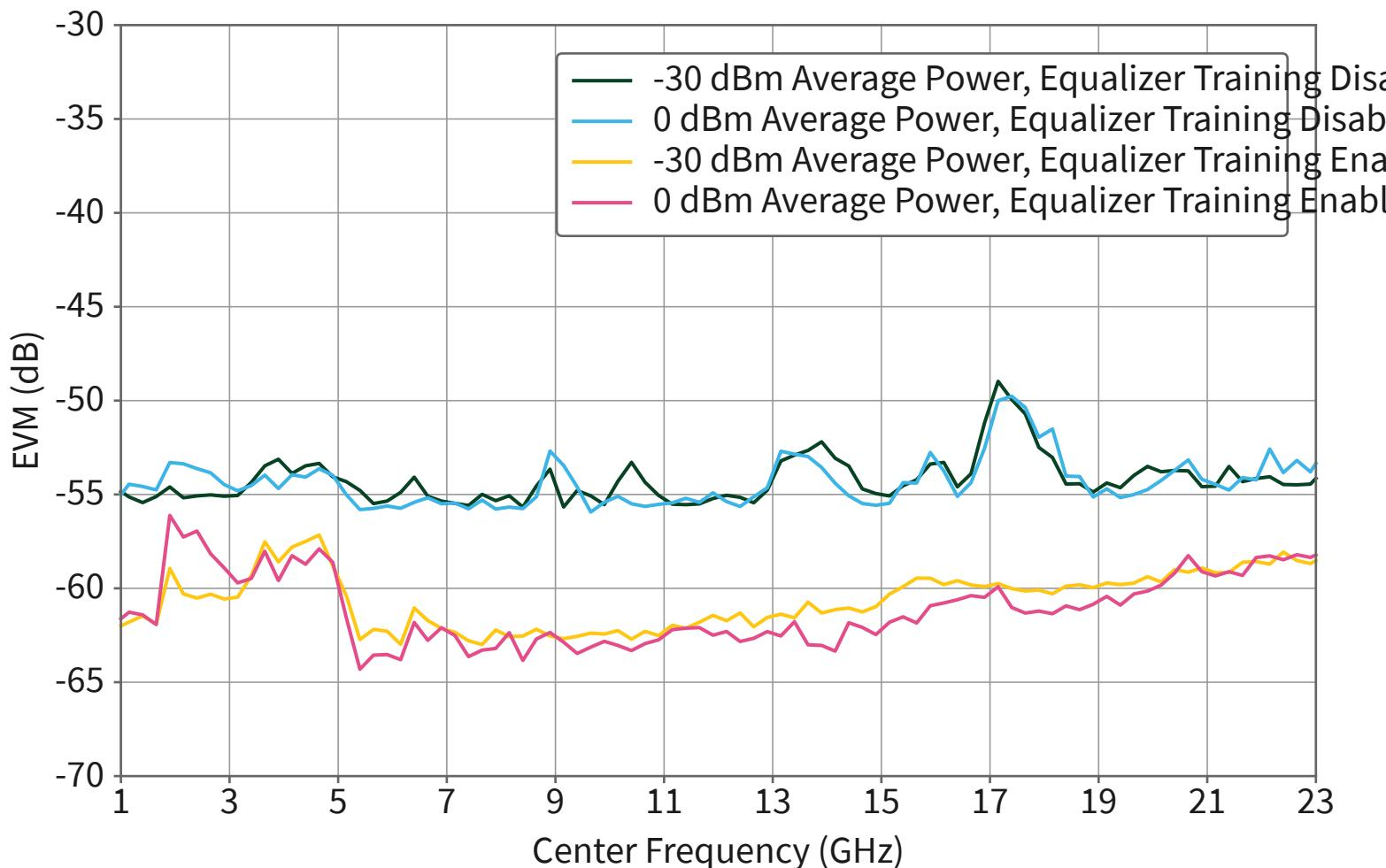
Conditions: RF OUT loopback to RF IN; 12.5 MHz bandwidth 64-QAM modulated signal; pulse-shape filtering: root-raised cosine, alpha = 0.25; PXIE-5842 RF input reference level and RF output power level set to value specified in legend; Offset Mode: Automatic; acquisition length: 300  $\mu$ s
