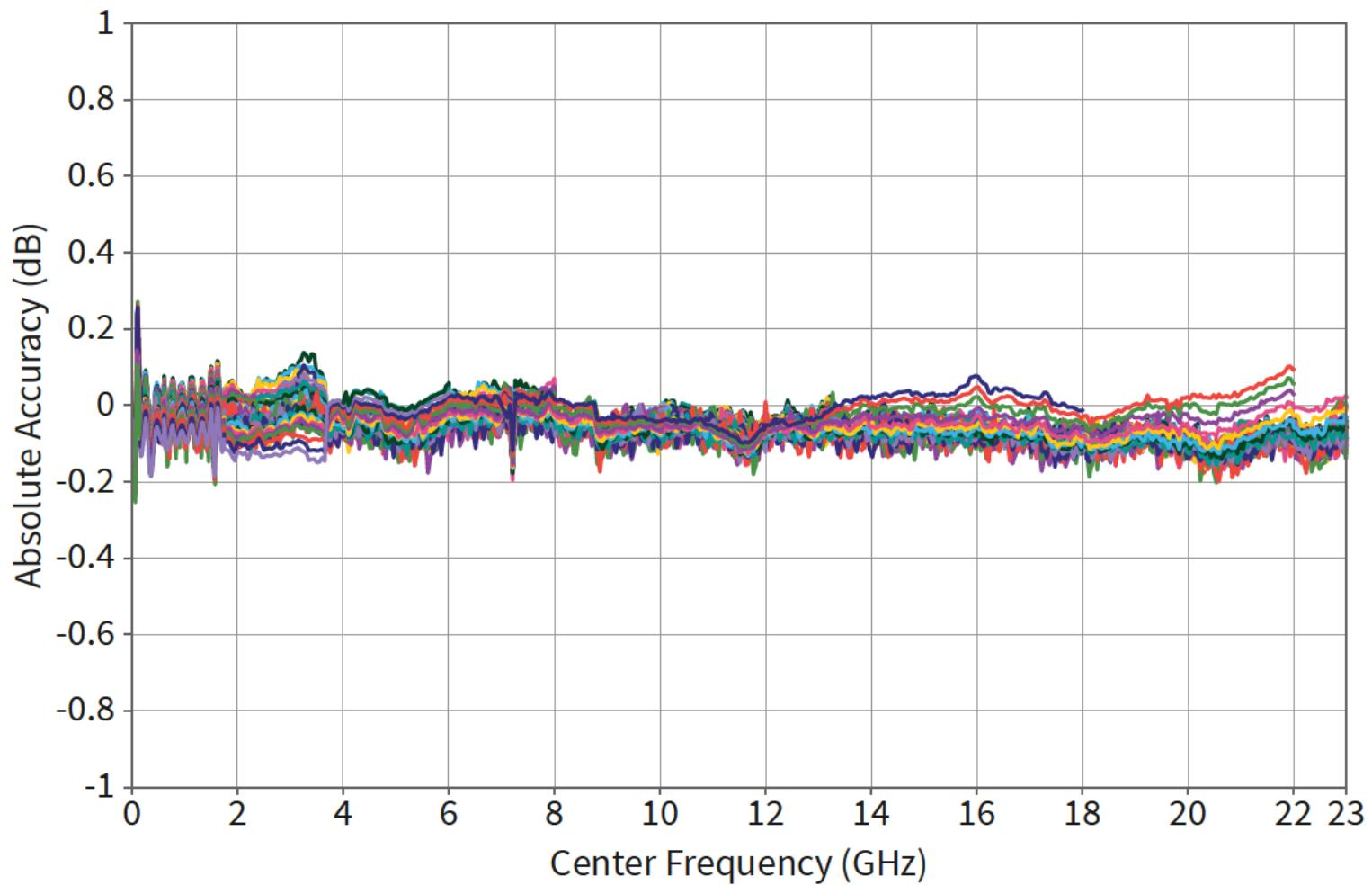
Conditions: Measured in 1 dB steps between -30 dBm and Maximum Leveled Power.
