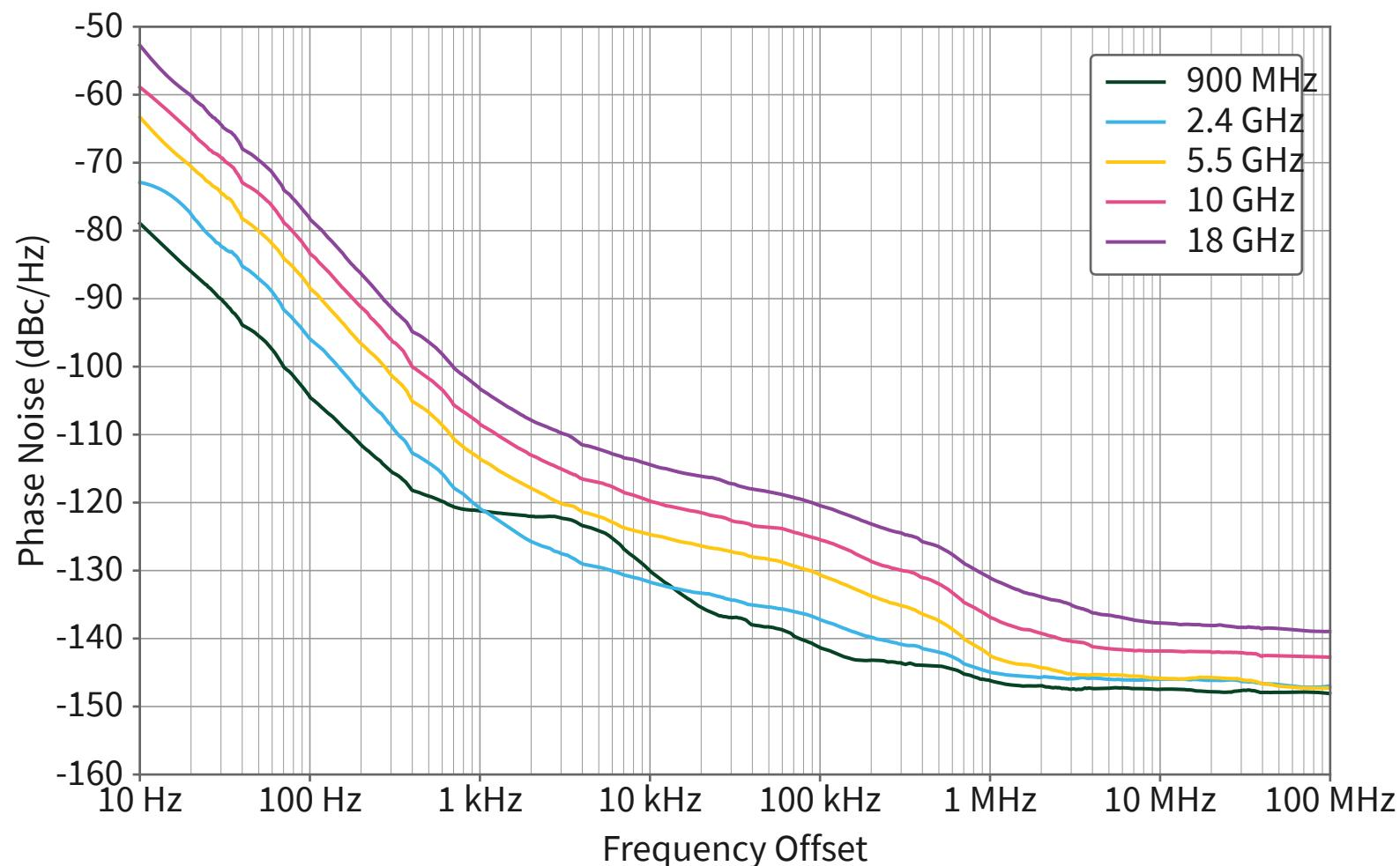
Measured data post-processed using Savitzky-Golay filter.
