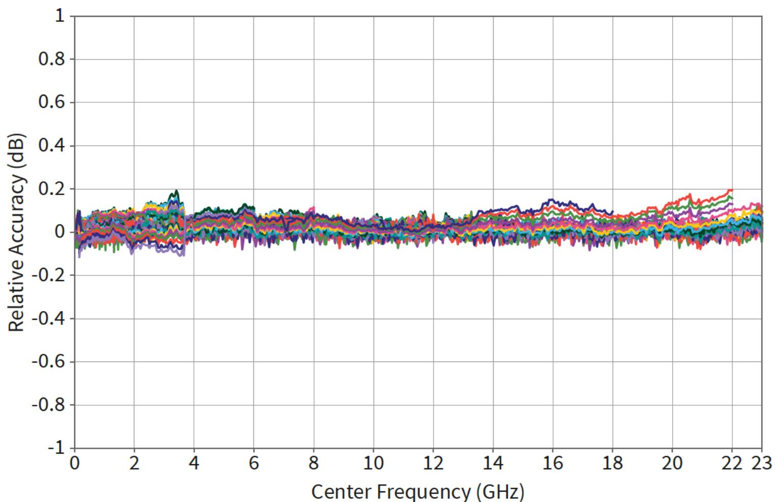
Conditions: Measured in 1 dB steps between -30 dBm and Maximum Leveled Power. Normalized to absolute accuracy at the 0 dBm Power Level Setting.
