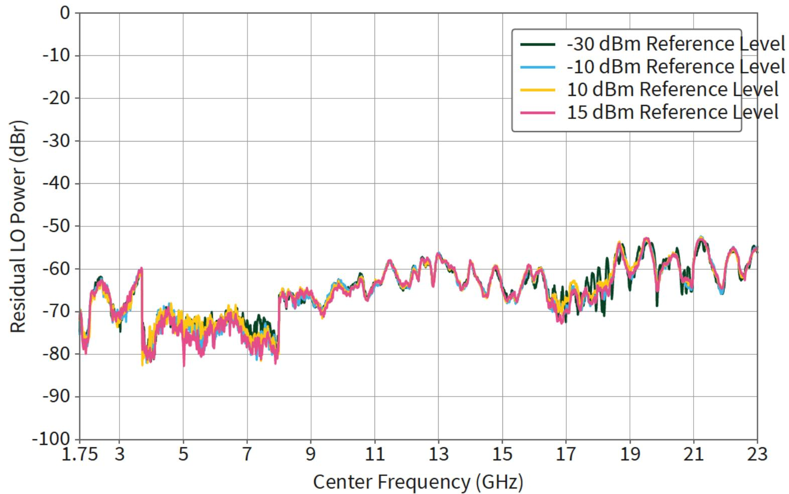
Conditions: Measured by sweeping a 0 dBm CW signal across the bandwidth and calculating the maximum residual LO power.
