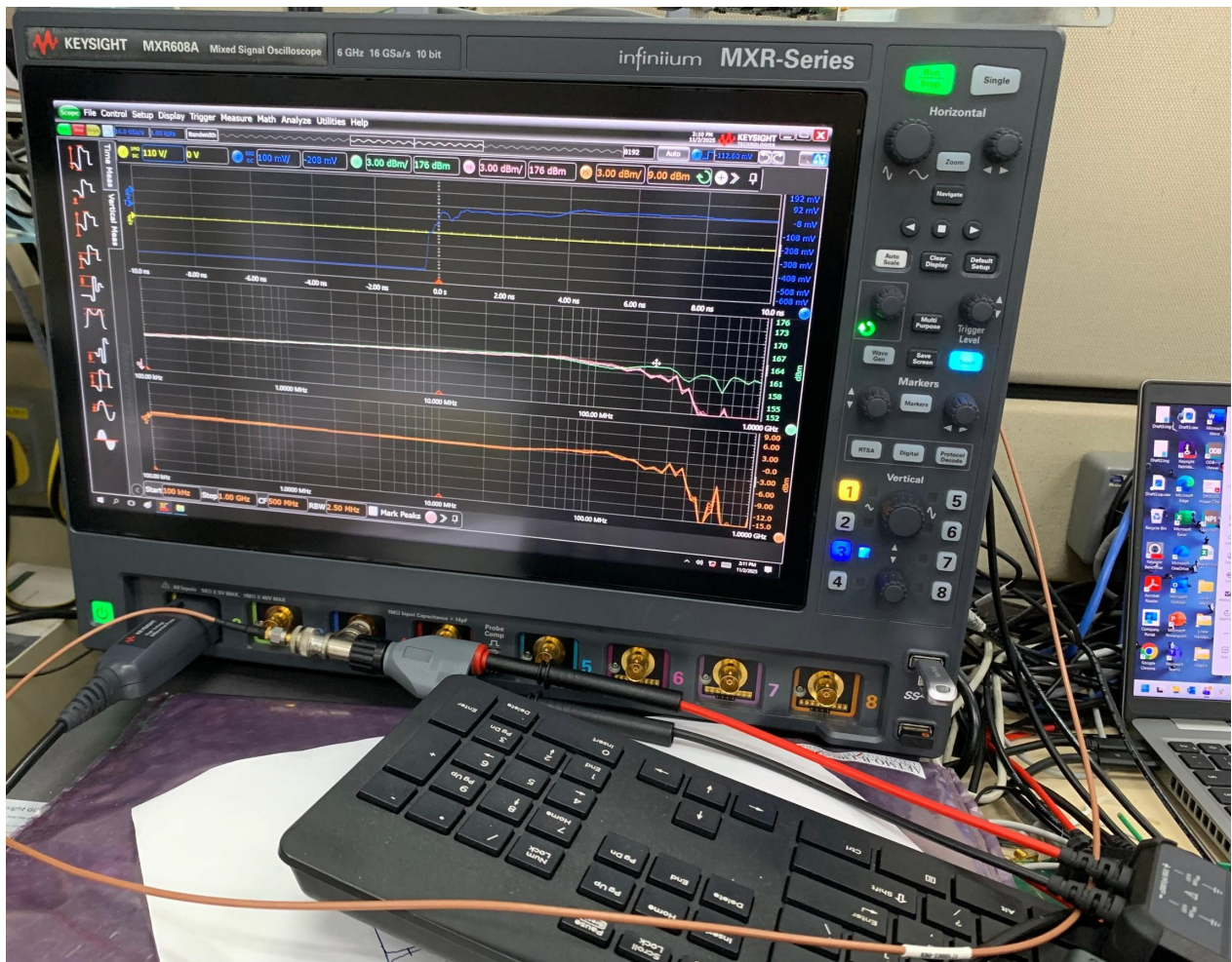
Figure 21 Connecting the probe with a BNC (Male) To Banana Jack Dual Adapter
