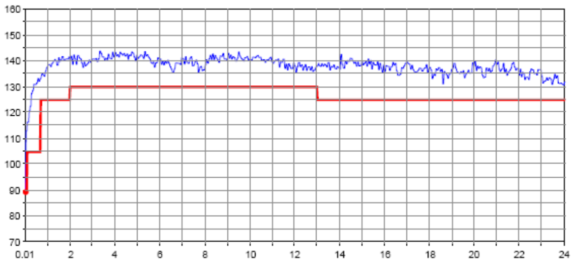
Dynamic range in dB versus frequency in GHz of the R&S®ZVA24
