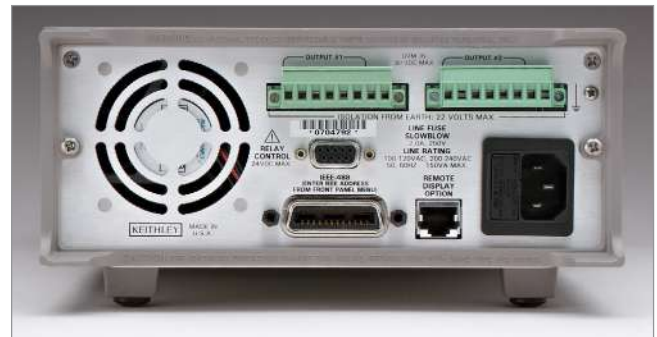
Figure 8. 2306 Rear Panel showing 8-position power output connectors, RJ-45 remote display connector, DB-9 relay output connector, IEEE-488 connector, and power input socket.
