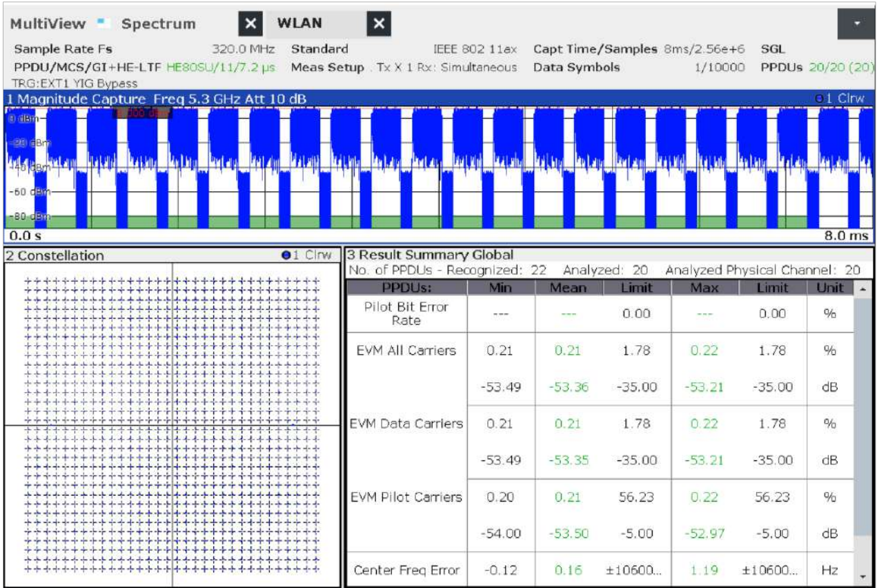
Measured EVM for an IEEE 802.11ax signal with 80 MHz bandwidth
