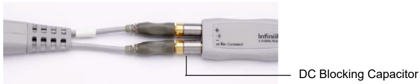
Figure 3 Placement of DC Blocking Capacitor Between a Probe Amplifier and a Probe Head
