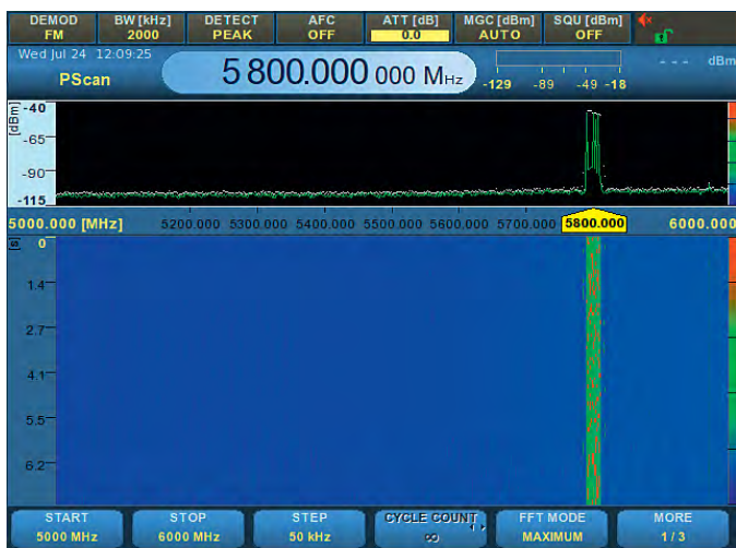
Detection of a hopper signal in the 5.8 GHz ISM band using the fast spectral scan over the 1 GHz bandwidth.
