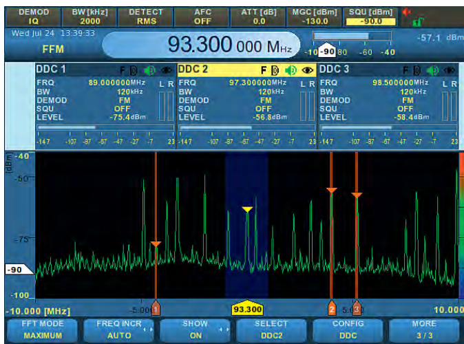
3+1 demodulation channels with different parameters within the realtime bandwidth.
