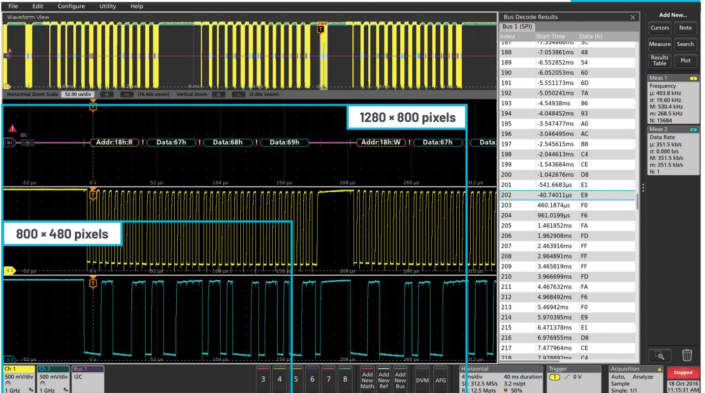
Display resolution on some competitors' products is as low as 800 × 480 pixels. That's less than 20% of the 1920 × 1080 pixel display resolution of the 3, 4, 5, and 6 Series products. Even larger 1280 × 800 pixel displays do not provide the same level of detail.
