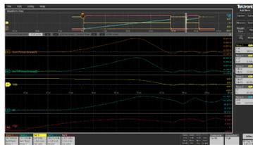
Double pulse test analysis package determines energy loss, reverse recovery and other key parameters on wide bandgap MOSFETs. Tektronix IsoVu™ probes enable accurate visualization of fast, floating signals on SiC and GaN devices.
