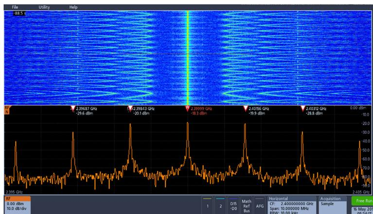
The Spectrogram display illustrates slowly moving RF phenomena. As the peaks change in both frequency and amplitude the changes are easy to see.
