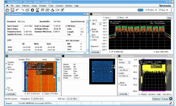
SignalVu-PC turns your Windows-equipped 5 or 6 Series MSO into a wideband vector signal analyzer. It can be customized to suit your application.
