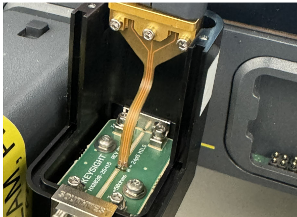
Figure 15 MX0041A probe head connected to DUT
