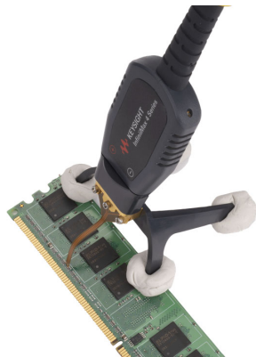
Correct securing method with InfiniiMax 4 probe amplifier and probe head secured using MX0046A vertical cradle and putty
