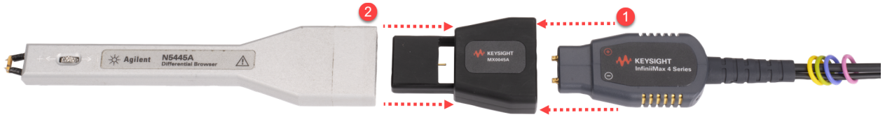
Figure 20 Order of connecting N5445A Probe Head & MX0032A Probe to MX0045A Adapter
