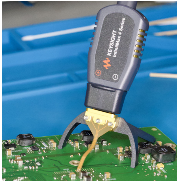
Figure 25 MX0041A probe head connected to probe head connector and vertical cradle
