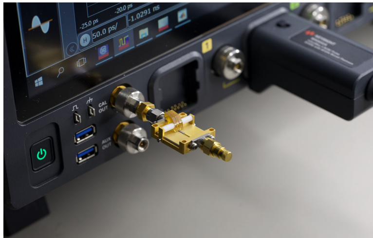
Figure 30 MX0104A deskew fixture connected to oscilloscope's Cal Out connector
