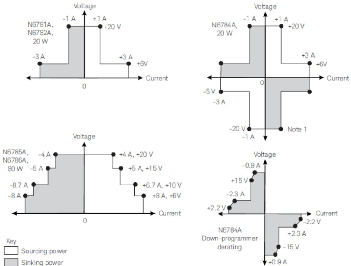
Note 1. When sinking power, the N6784A model can operate at the maximum rated output power for only a limited amount of time. The unit monitors the temperature of the internal power devices and latches the output off if the output power has exceeded its safe limits. A protect clear is required to resume normal operation. The condition is annunciated by the OT status bit. Refer to the down programmer derating figure for the values of the safe limit boundaries.
