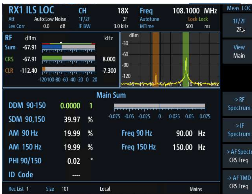
Figure 4-2: ILS Localizer mode main results view
