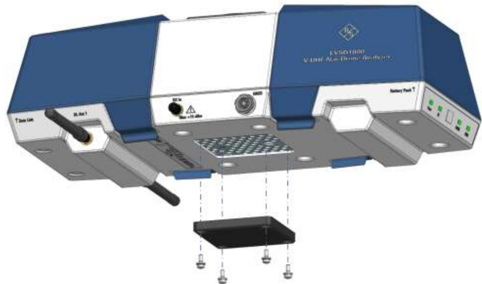
Figure 1-5: Removing the protection cover from the bottom panel
