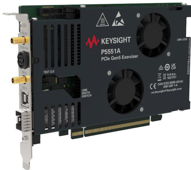
Figure 1. P5551A PCIe 5.0 Protocol Exerciser
