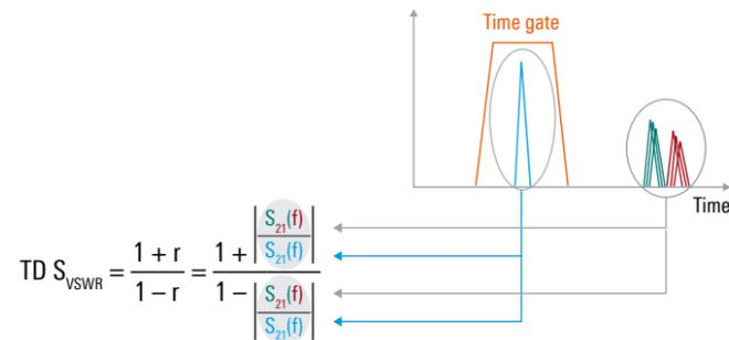
The time domain site VSWR (TD  $S_{VSWR}$ ) measurement in line with ANSI C63.25 is a fast and precise method for validating fully anechoic rooms (FAR). It involves a series of impulse response measurements, which are performed by a 2-port R&S®ZNB20 or R&S®ZNB26 equipped with the R&S®ZNB-K2 option, plus an R&S®HF907 double-ridged waveguide horn antenna. The R&S®ZNRUN software can be used to automate the test sequence.
