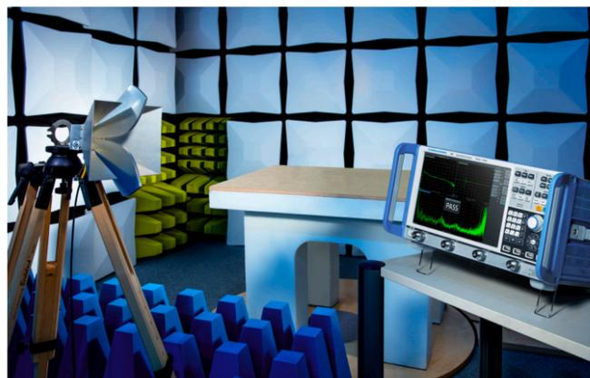
R&S®ZNB20 equipped with the R&S®ZNB-K2 time domain analysis option, together with an R&S®HF907 double-ridged waveguide horn antenna, provides an ideal solution for fast and accurate site validation measurements using the TD  $S_{VSWR}$  method in line with ANSI C63.25.
