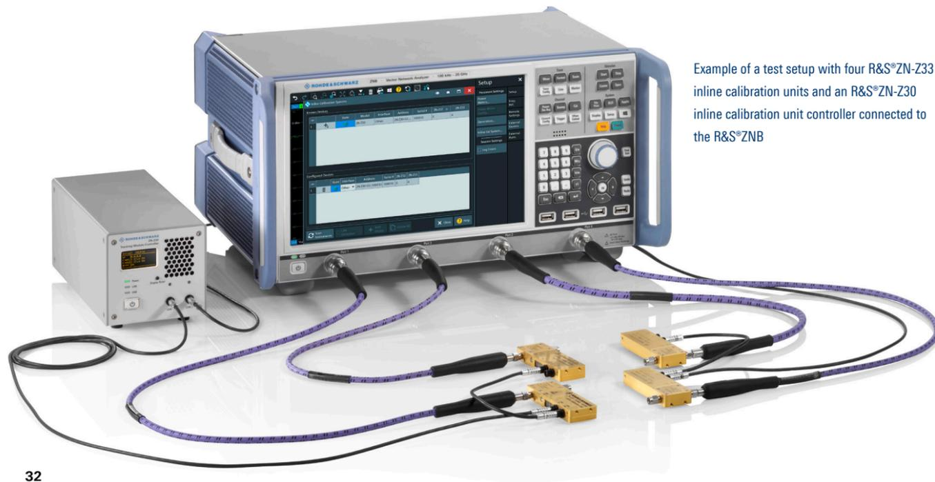
Example of a test setup with four R&S®ZN-Z33 inline calibration units and an R&S®ZN-Z30 inline calibration unit controller connected to the R&S®ZNB
