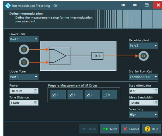
Configuring mixer measurements with a DUT-centric wizard
