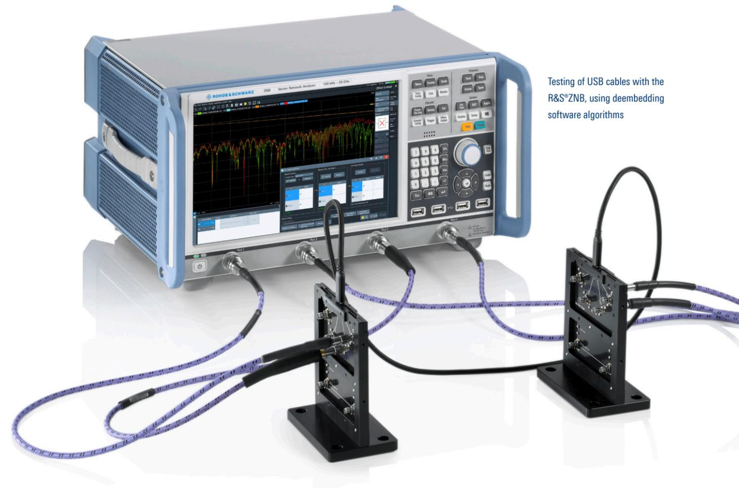
Testing of USB cables with the R&S®ZNB, using deembedding software algorithms
