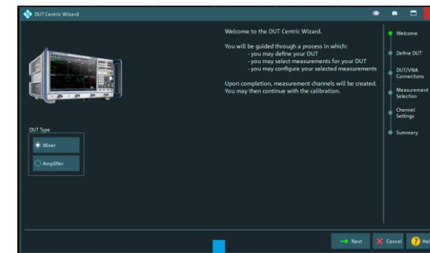
Based on the selected type of DUT, the wizard guides the user step by step to the desired measurement setup.
