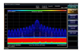
4051 can achieve seamless Real-time Spectrum Analysis, and frequency template trigger function, which can be used to trigger, capture, and analyze complex signals.
