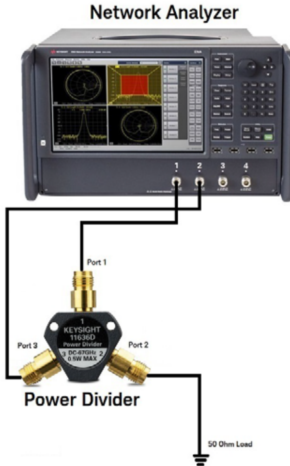
Figure 3-4 Output tracking test setup (Port 2 Terminated)
