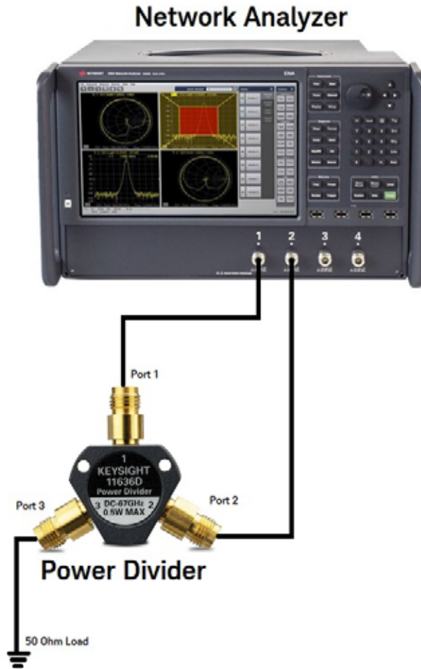
Figure 3-2 Input return loss test setup
