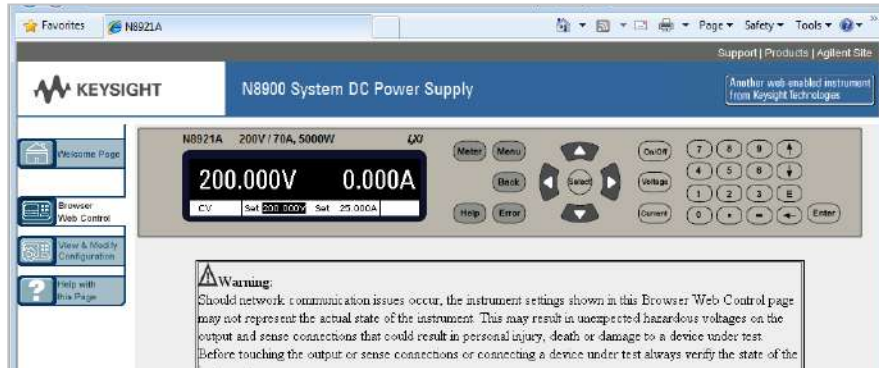
Figure 3. N8900 Series web graphical user interface for remote access and control of the power supply
