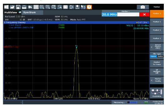
Figure 8-3: Example for an upper limit line
