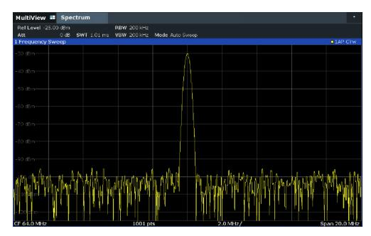
Figure 4-6: Calibration signal with optimized display settings
