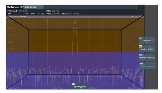
Figure 4-7: Adding a Spectrogram to the display
