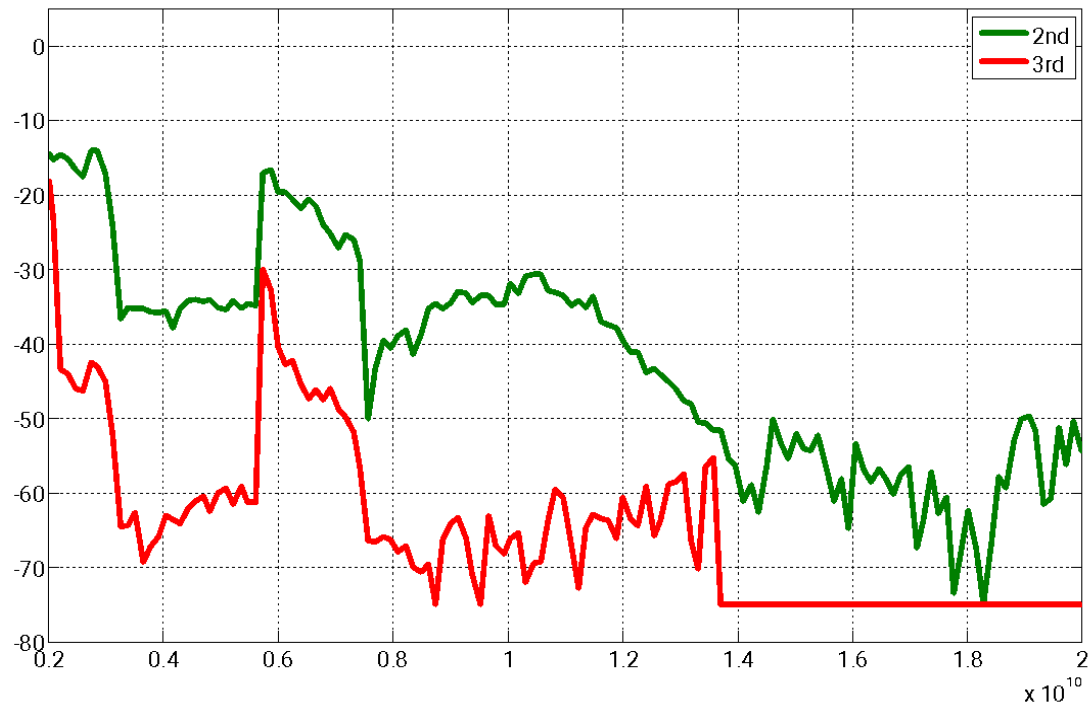
Figure 2. Harmonic performance at 0 dBm — Harmonic output power [dBc] vs. frequency [Hz]
