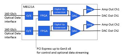
For modulation bandwidths up to approximately 250 MHz, the PCI Express interface to a host PC can be used to stream data into the AWG in a future release.<sup>1</sup>
