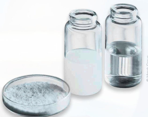
Fig. 4: Thermotropic liquid crystals change their phase depending on the temperature. At the melting point T_m , the crystalline material passes into the nematic phase and turbidity sets in. At the transparency point T_c , the uniform orientation of the molecules is lost and the liquid becomes transparent. One current research objective is to create liquid crystal mixtures with the greatest possible \Delta\epsilon , which expresses their “tunability”.
