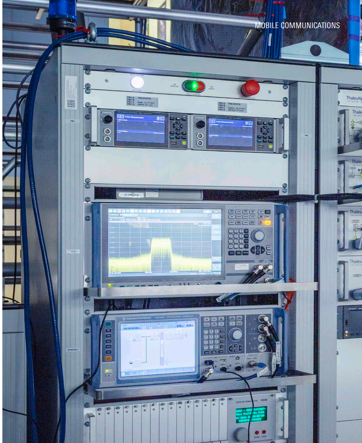
Fig. 5: Satellite manufacturer Thales Alenia Space uses the R&S®SMW200A signal generator and the FSW signal and spectrum analyzer to test 5G NTN infrastructure compo- nents in Madrid.
