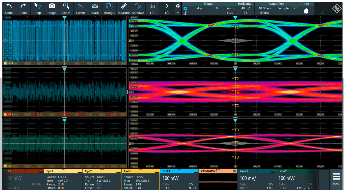
Fig. 3: Comparison of waveforms and eye patterns at different test points for a USB 3.2 Gen 1 signal (5 Gbit/s):
