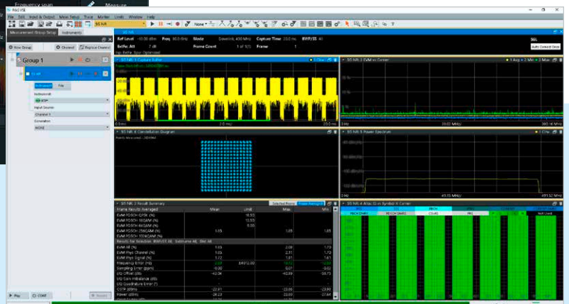
Fig. 6: 5G analysis at 80.0 GHz using R&S®VSE vector signal explorer software.
