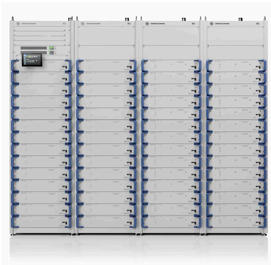
Fig. 2: The R&S®TE1 is designed for modular expansion of transmit power using a rack system. Each cabinet has space for up to 14 racks for 24.5 kW of total transmit power.
