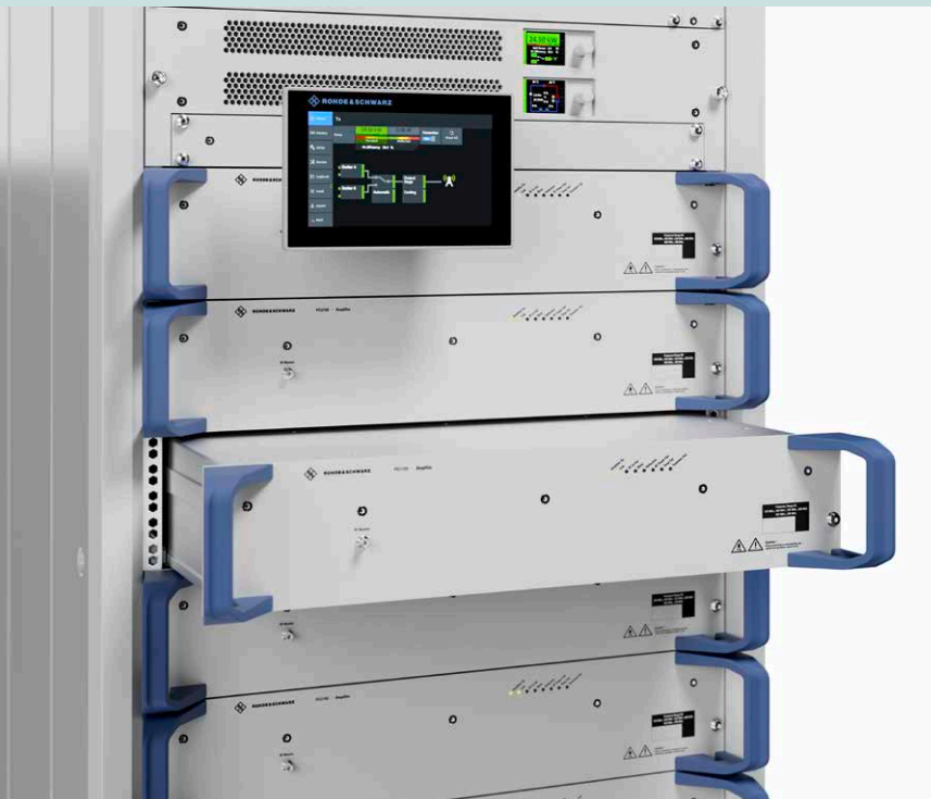
Fig. 2: The R&S®TE1 is designed for modular expansion of transmit power using a rack system. Each cabinet has space for up to 14 racks for 24.5 kW of total transmit power.
