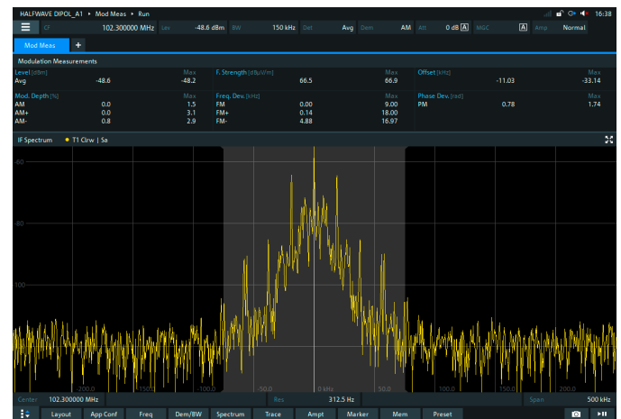
ITU-compliant measurements of AM depth, FM deviation and PM deviation in a single view
