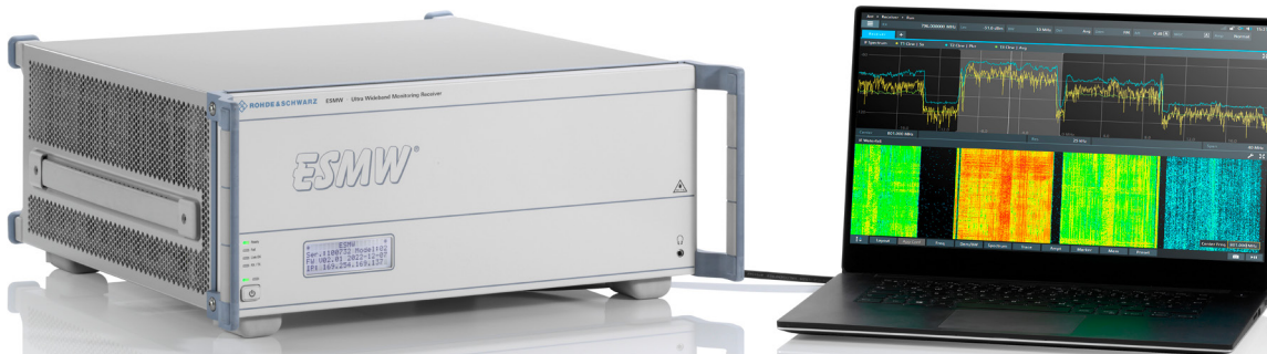
LAN remote control using the R&S®ESMW GUI running on a Windows laptop
