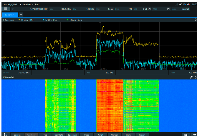
500 MHz real-time bandwidth with up to three configurable spectrum traces
