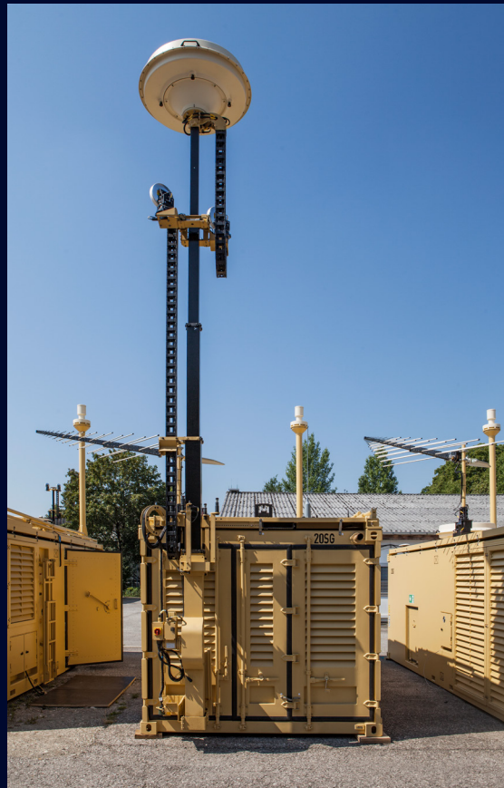
R&S®ESMW installed in a COMINT shelter
