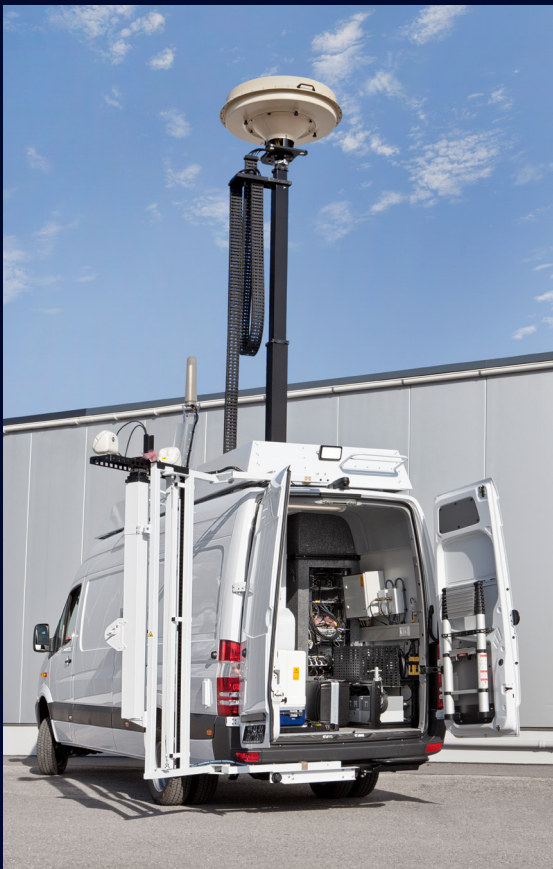
R&S®ESMW installed in a mobile monitoring station
