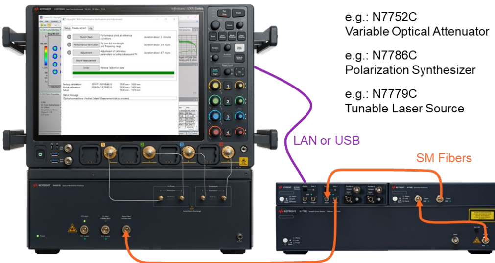
Figure 2. On-site performance verification and adjustment setup
