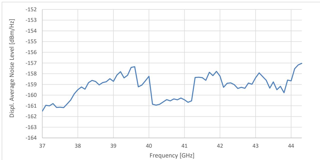
Measured at R&S®CMXHEAD30 remote radio head, RF1: displayed average noise level from 37 GHz to 44.3 GHz
