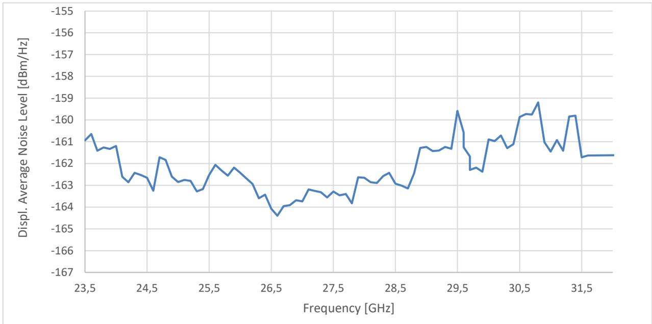
Measured at R&S®CMXHEAD30 remote radio head, RF1: displayed average noise level from 23.5 GHz to 31.8 GHz
