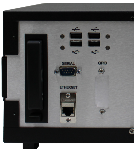
Rear panel removable drive and input/output connectivity
