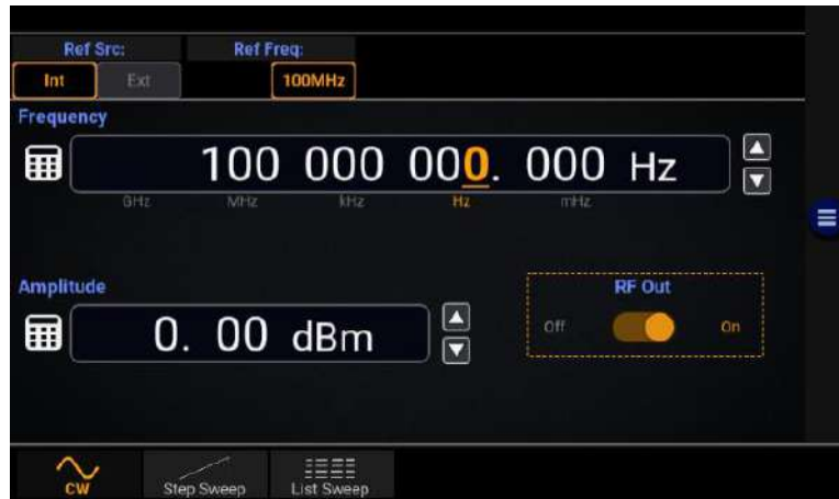
Figure 3-5. SGX1000 CW Operation Mode Generating a 100 MHz signal.
