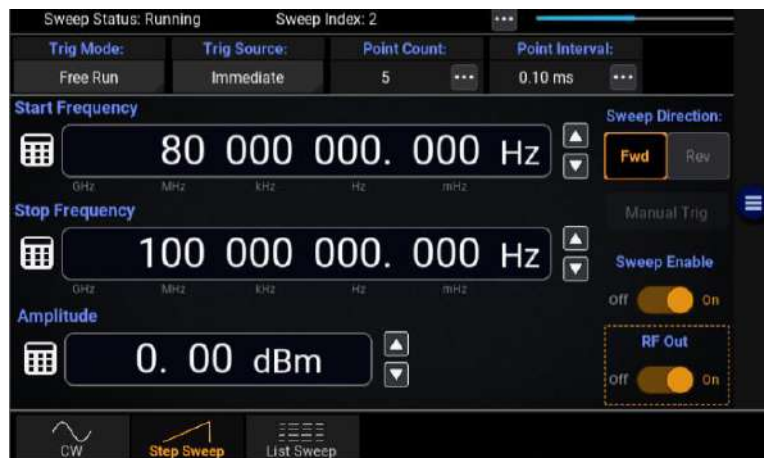
Figure 3-6. Step Sweep Screen Showing a Sweep From 80 MHz to 100 MHz
