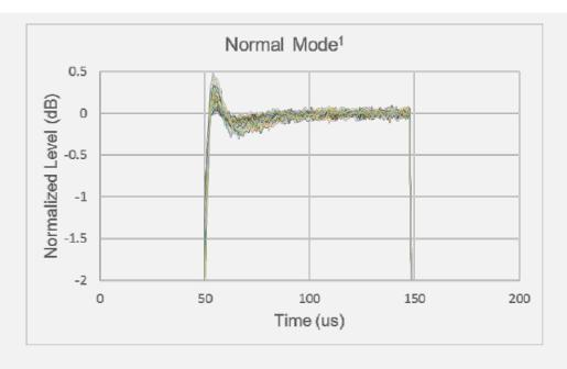
Measured with a 500 kHz IF bandwidth, averaging factor of 16 (Average Type = Point). With 100 us pulse width setting. 50 usec/div.
