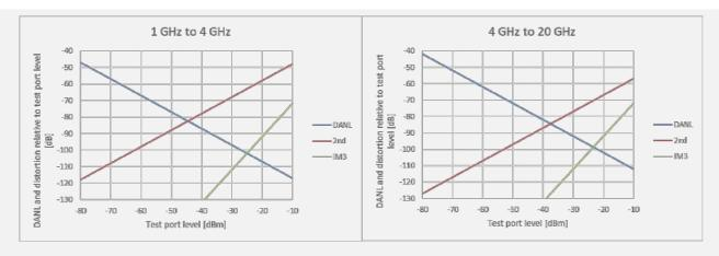
1. With High Attenuation. 2<sup>nd</sup> harmonic distortion applies up to 10 GHz.
