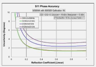
Table 4. M9800A, M9801A, M9802A, M9803A or M9804A with N4691D Electronic Calibration (ECal) Module with Option 0DC
