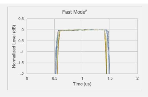
2. Measured with a 15 MHz IF bandwidth, averaging factor of 16 (Average Type = Point). With 1 us pulse width setting. 500 nsec/div.
