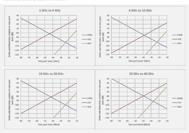
2. With High Attenuation. 2<sup>nd</sup> harmonic distortion applies up to 26.5 GHz.
