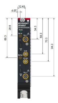
Dimensions (front view, M9800A/01A/02A/03A/04A/05A/06A/07A/08A with option 200, in millimeters)
