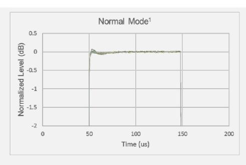
1. Measured with a 500 kHz IF bandwidth, no averaging (Average Type = Point). With 100 us pulse width setting. 50 usec/div.
