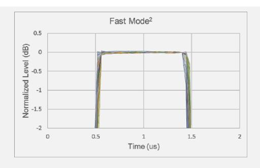
Measured with a 15 MHz IF bandwidth, averaging factor of 16 (Average Type = Point). With 1 us pulse width setting. 500 nsec/div.
