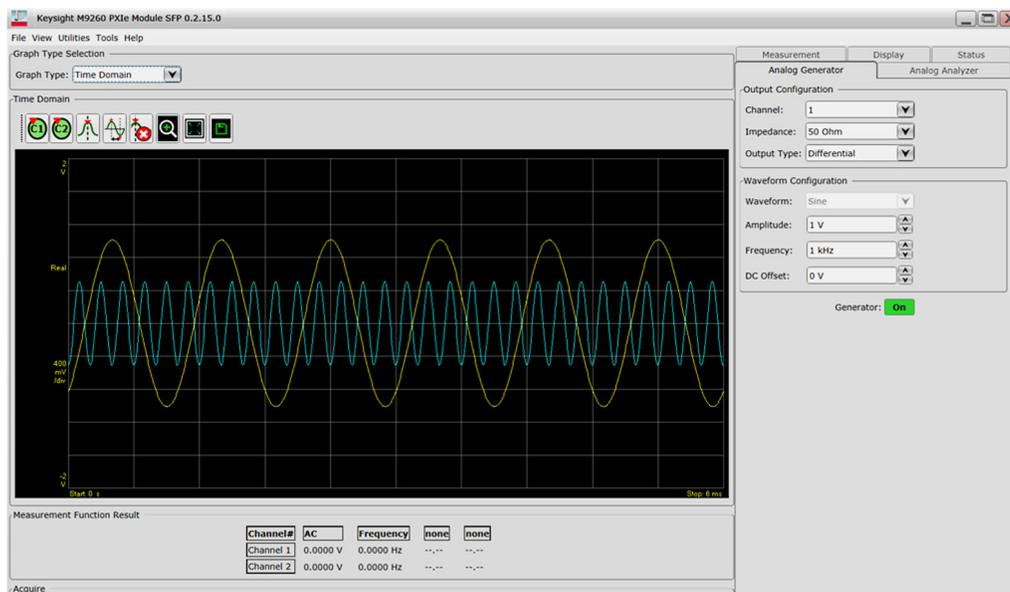
Figure 4. M9260A PXIe module soft front panel interface
