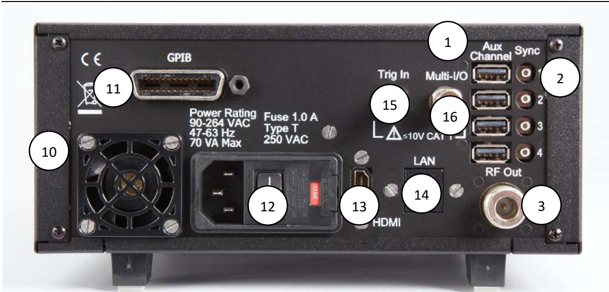
Figure 3-2. PMX40 RF Power Meter - Rear Panel
